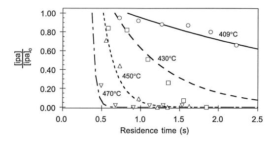
Figure 5 Comparison of calculated first order reaction kinetics (lines) to isopropanol experimental data (open symbols) for runs 2 (409°C) $\bigcirc$ —, 4 (430°C) $\square$ — – , 6 (450°C) $\triangle$  – – – , and 8 (470°C) $\nabla$  — – – .
