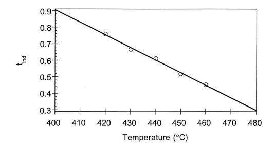
**Figure 4** Measured induction times for isopropanol destruction (runs 3-7) plotted versus temperature (the line is calculated from a linear least squares fit of the data).
