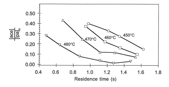
Figure 6 Measured acetone concentration plotted versus residence—time for conditions when the normalized isopropanol concentration is less than 0.1, runs 6 (450°C) $^{\circ}$ , 7 (460°C) $^{\circ}$ , 8 (470°C) $^{\circ}$ , and 9 (480°C) $^{\circ}$ .
