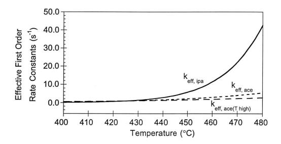
Figure 8 Comparison of the calculated effective first order rate constants for the oxidation of isopropanol,  $k_{eff, ipa}$ , and acetone (using two different fitting methods)  $k_{eff, ace}$  and  $k_{eff, ace(T \ high)}$  — - .
