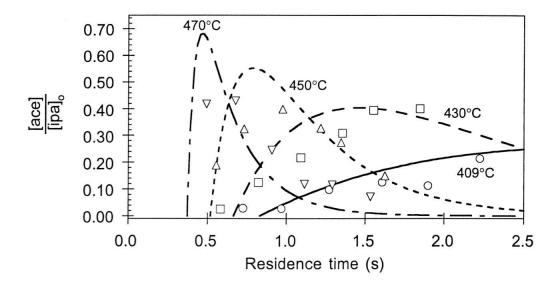
Figure 7 Comparison of calculated first order reaction kinetics (lines), to acetone experimental data (open symbols) for runs 2  $(409^{\circ}C)^{\circ}$ , 4  $(430^{\circ}C)^{\square}$  – – , 6  $(450^{\circ}C)^{\triangle}$  – – – , and 8  $(470^{\circ}C)^{\triangledown}$  – – .
