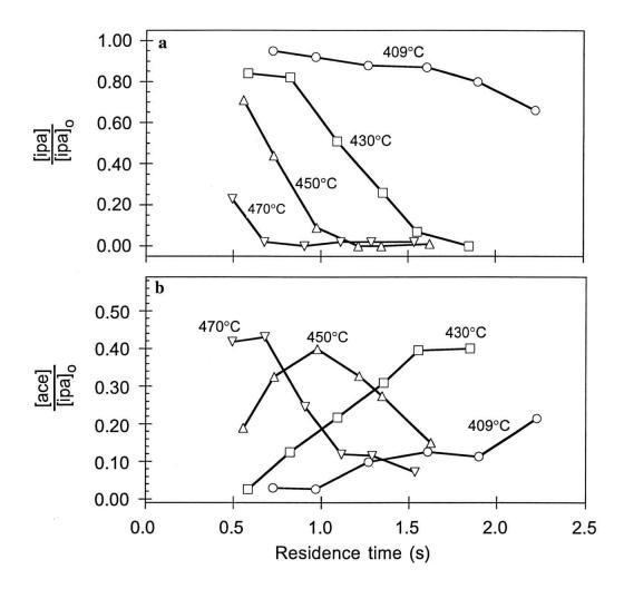
Figure 2 Measured normalized species concentration profiles plotted versus residence–time for (a) isopropanol and (b) acetone, runs 2 (409°C) $^{\circ}$ , 4 (430°C) $^{\Box}$ , 6 (450°C) $^{\triangle}$ , and 8 (470°C) $^{\nabla}$ .
