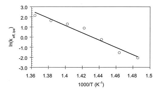
Figure 3 Effective first order rate constants for isopropanol destruction (runs 1-7) plotted versus 1000/T (the line is calculated from a linear least squares fit of the data).
