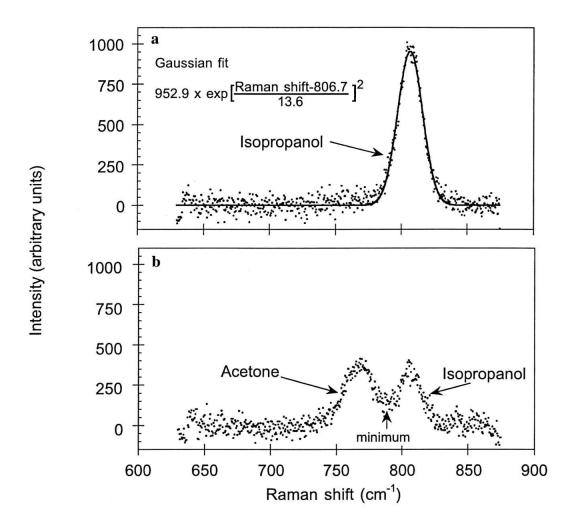
Raman spectra for run 3 (420°C). (a) At a short residence–time, 0.63 s, very little isopropanol has oxidized and no acetone has been produced, therefore, only an isopropanol peak is visible, a Gaussian fit is also shown. (b) At a longer residence–time, 2.0 s, both the isopropanol and acetone peaks are visible.
